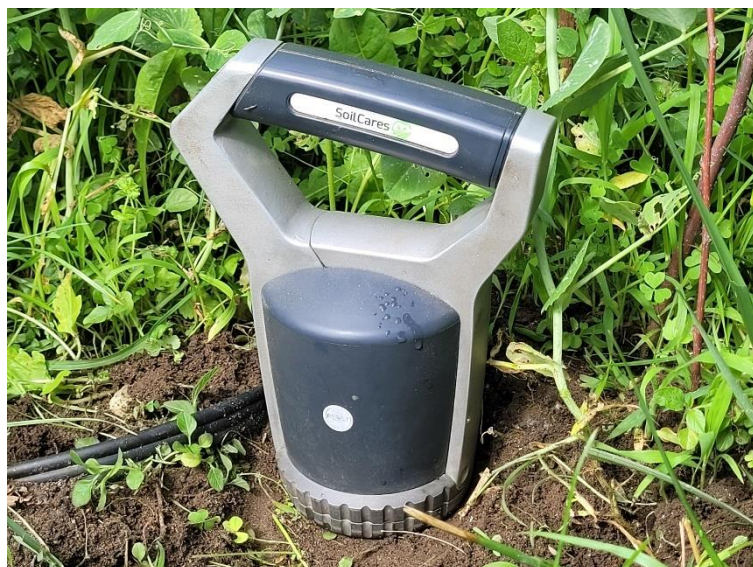
Figure 3: The NIR soil scanner in a garden environment during in situ measurements
