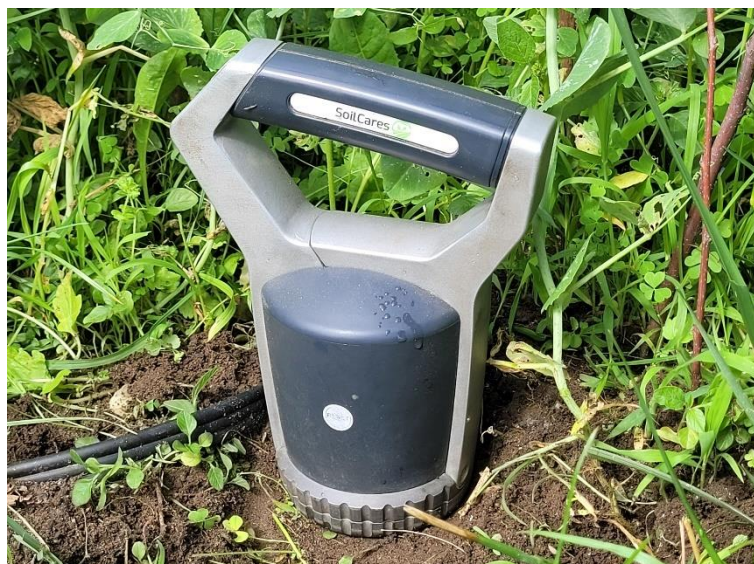
Figure 2: The NIR soil scanner in a garden environment during in situ measurements
